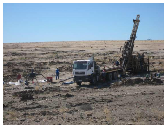
Figure 3: RC drilling at the northern end of Rossing South Zone 1. Note the outcrop increases to the left of the image (north) and the flat desert plain to the right (south).
