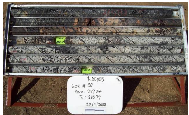
Figure 4: Rossing South Zone 2 drill core from RDD005.
