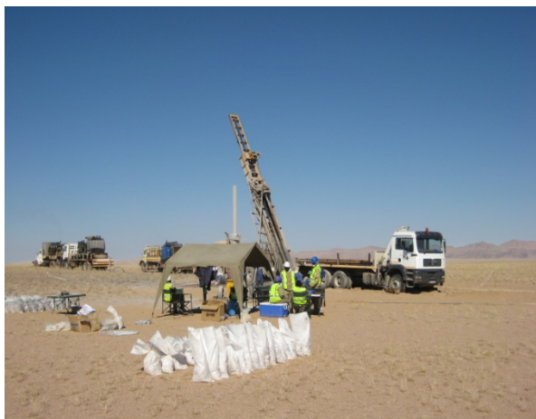
Figure 4: RC drill rig at Rossing South.
